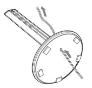
2 Thread the speaker cord through the post of the speaker stand, and connect it to the speaker. Make sure that the hole on the back of the speaker is in the right direction, as illustrated below.
